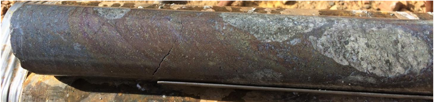
Figure 6: Massive sulphide interval from GLPD001
