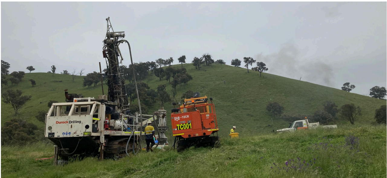
Image 1: RC 650 track mounted drill rig onsite at the Mantons Prospect located at Gundagai North
