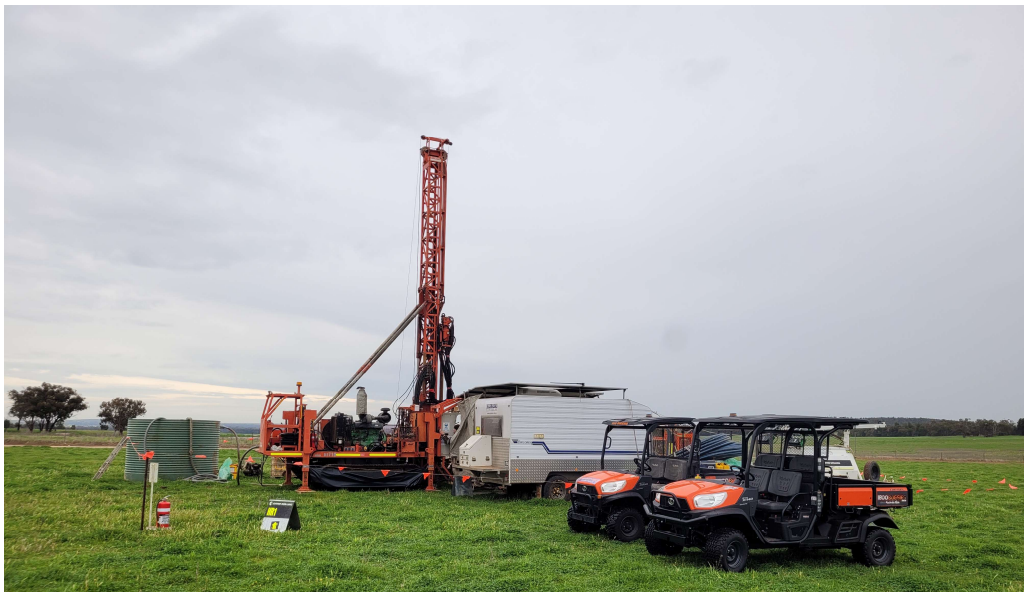
Image: Diamond drill rig on site and operational at the Narraburra Rare Earth Project
