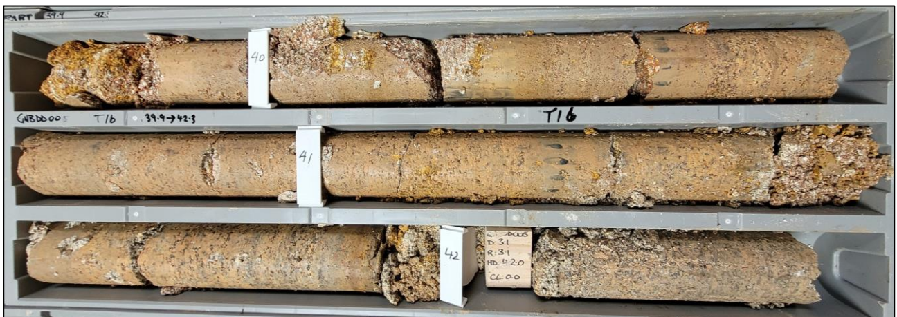
Image: Core from GNBDD005 (between 39-43m) containing TREO of up to 1218 ppm (weathered zone)
