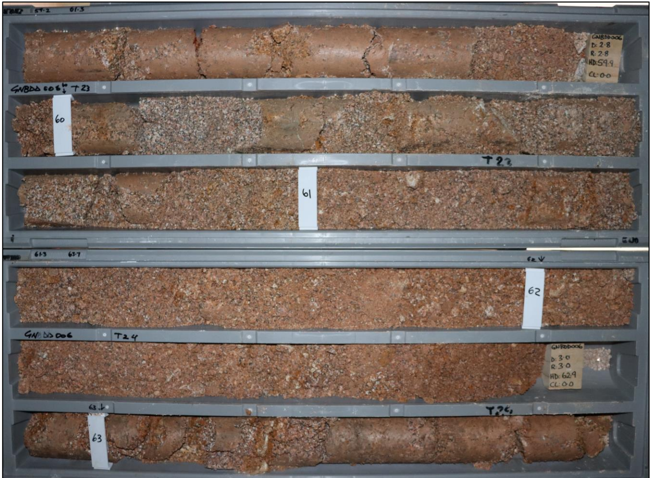
Image: Core from GNBDD006 (between 59-64m) containing TREO of up to 695 ppm (weathered clay material zone)
