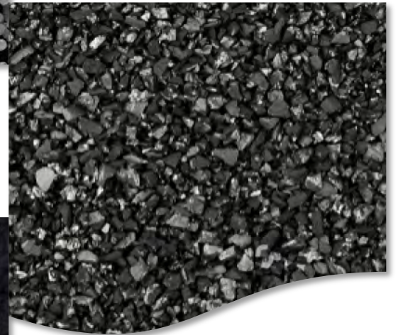
Granular activated carbon (GAC)
