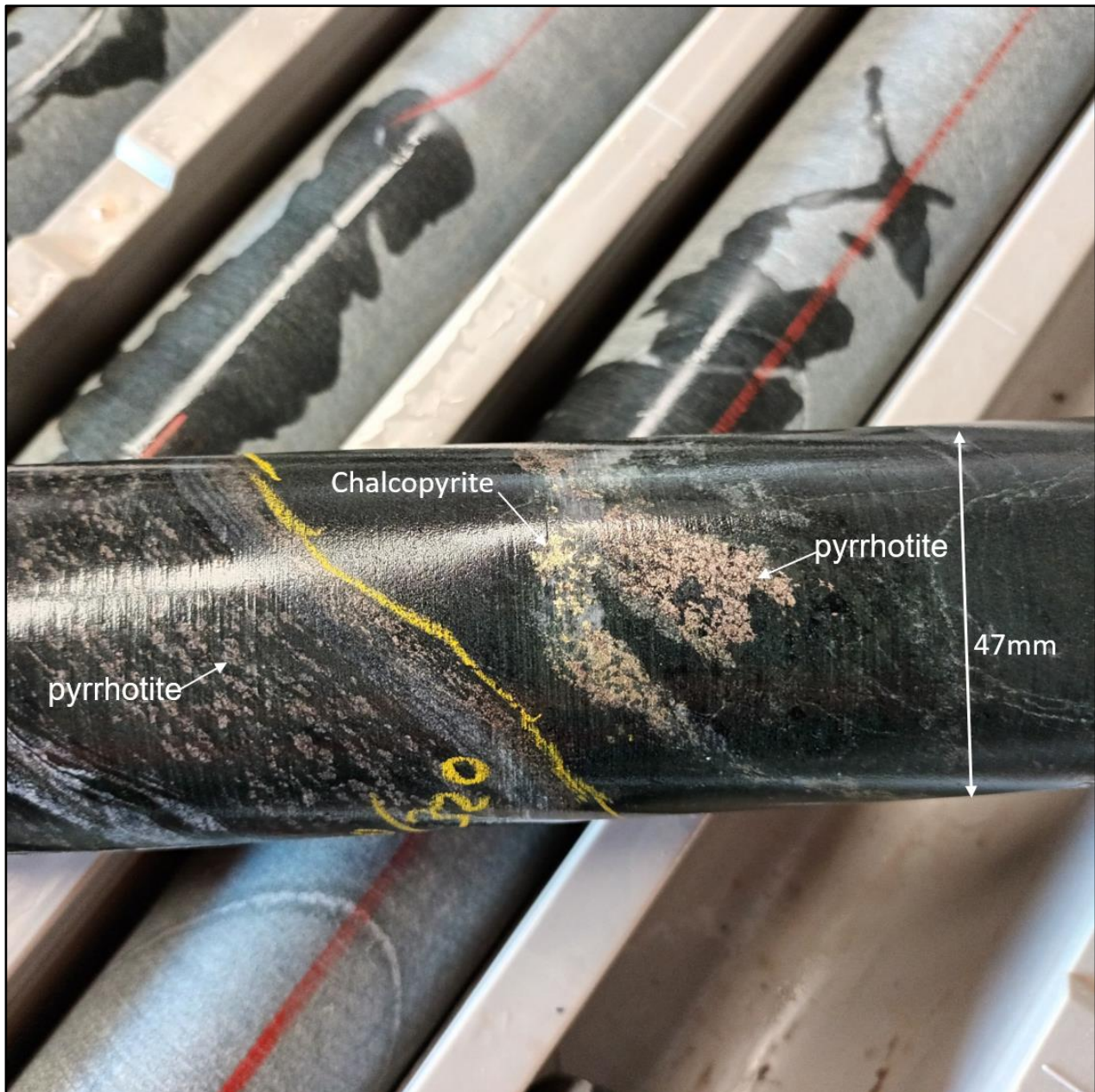
Figure 3 Close up image of sulphides intersected at 304.8m downhole.
