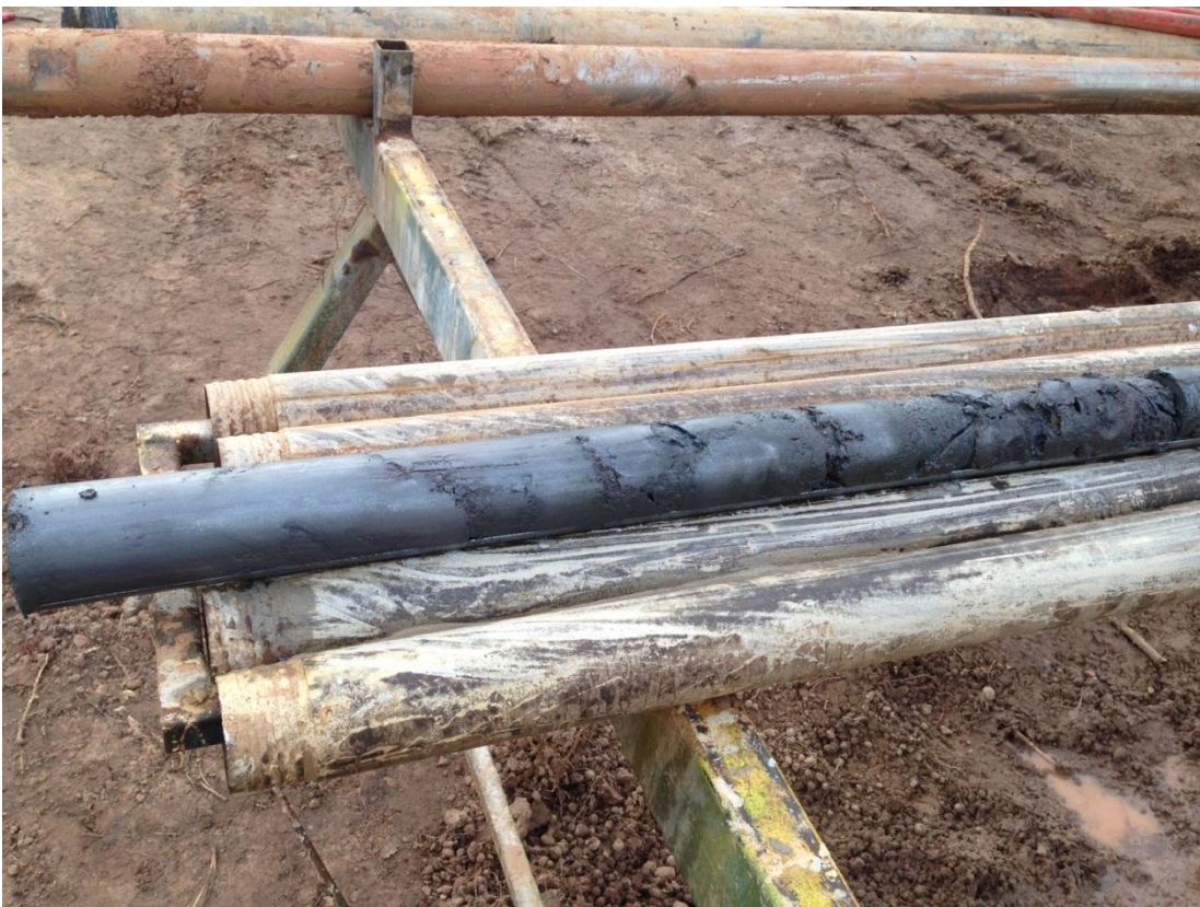
Figure 5 – MCDD004: Core from 51.1 m – 53 m Interval (34.9% TGC)
