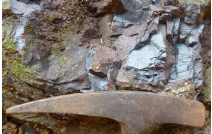
High grade outcrop from Youkou , 64% Fe reading from Niton XRF
