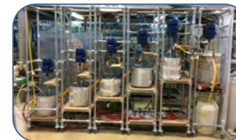
Neutralisation & Precipitation Circuit – Hydromet - ANSTO
