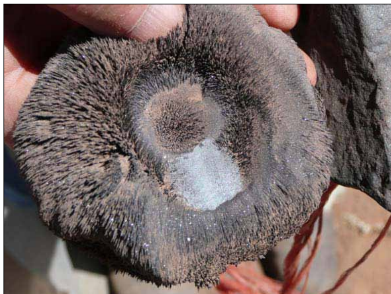
Coarse-grained magnetite drill chips from Lilydale on hand magnet
