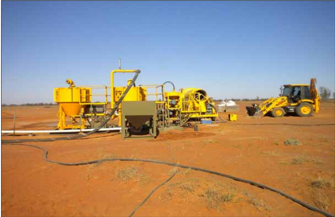
Gravity test plant at Portia
