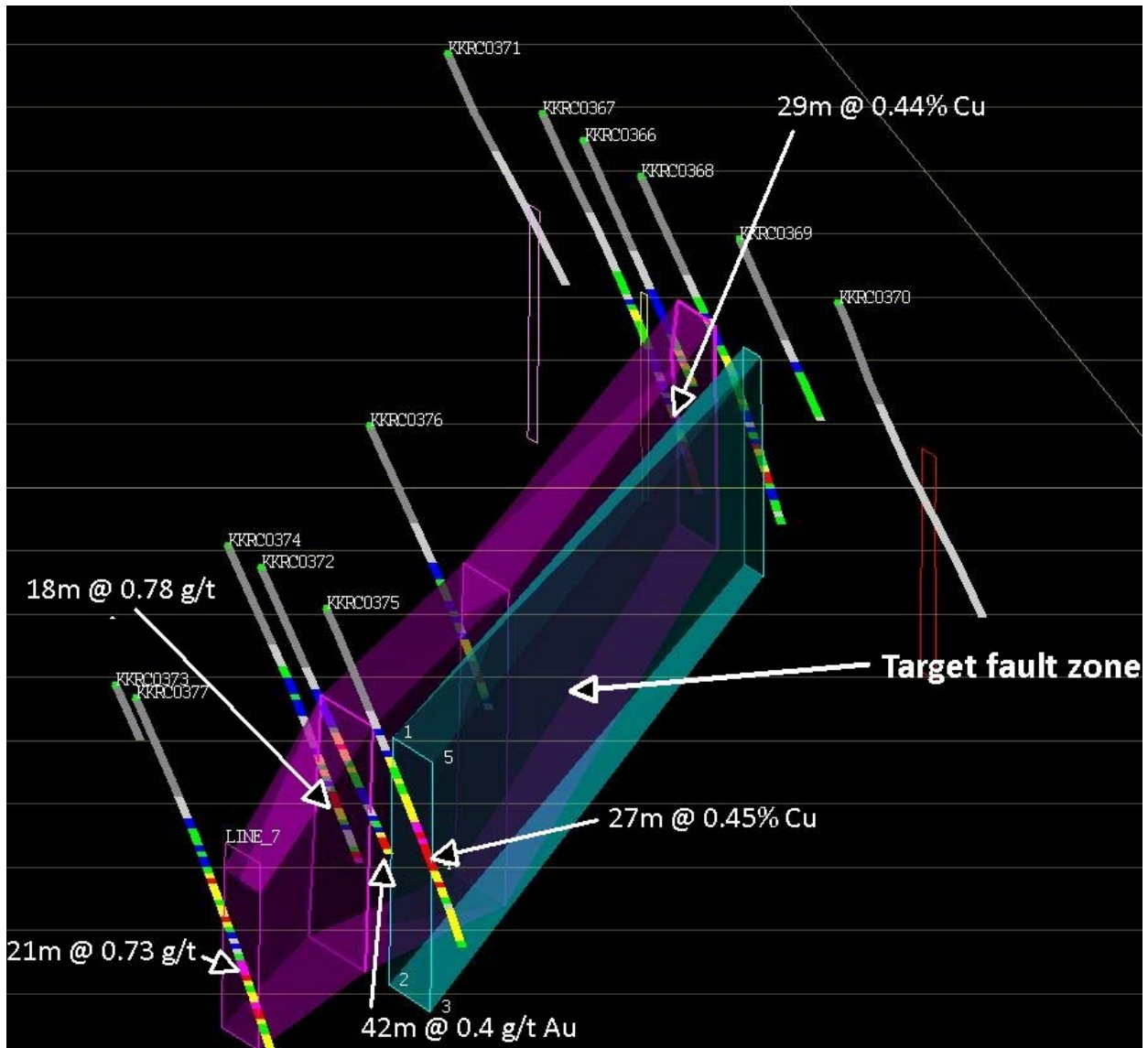
Drill intersections reported to date within the intensely quartz veined Kalkaroo north fault zone
