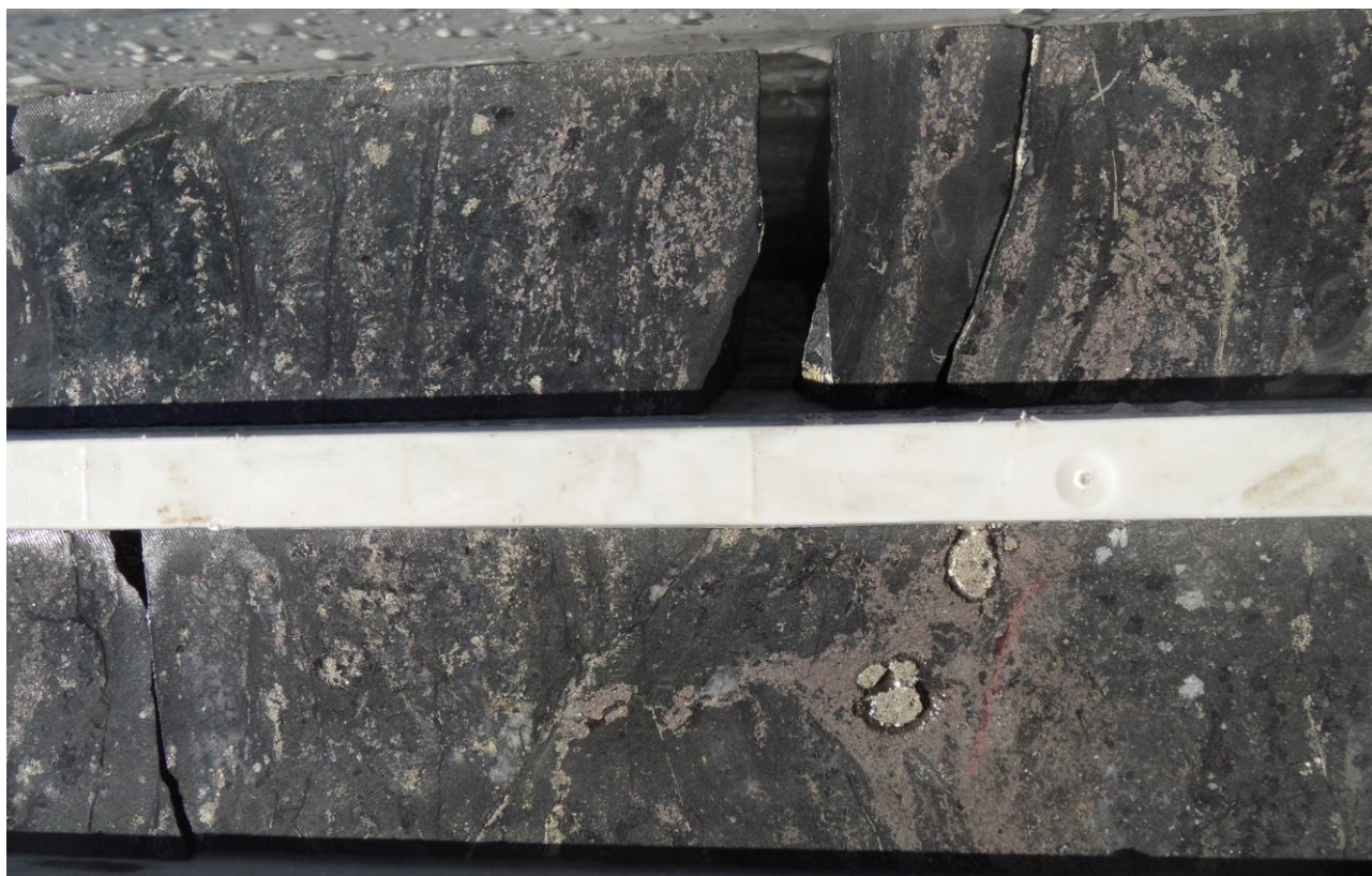
Skarn rocks in drillcore from Croziers Dam prospect, with abundant sulphide minerals including chalcopyrite (copper ore), magnetite (grey), pyrrhotite (bronze) and other dark greenish calc-silicate minerals.
