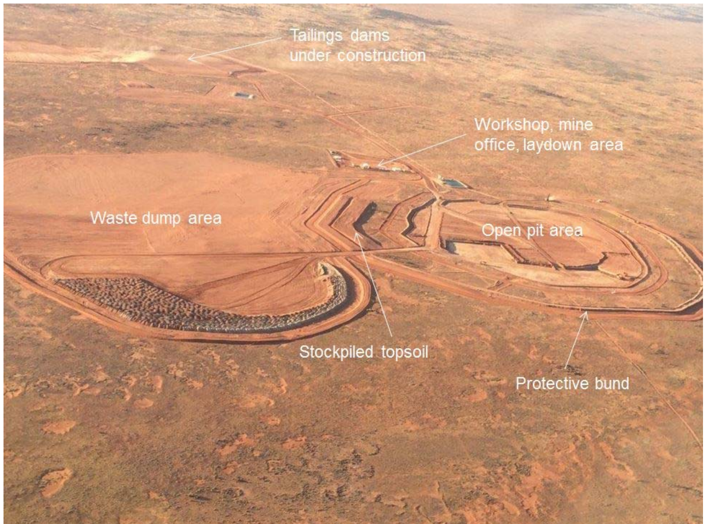
Aerial view of the Portia open pit taken earlier in the week, showing the extent of site works and current stage of excavation in the open pit. View direction is towards the north.
