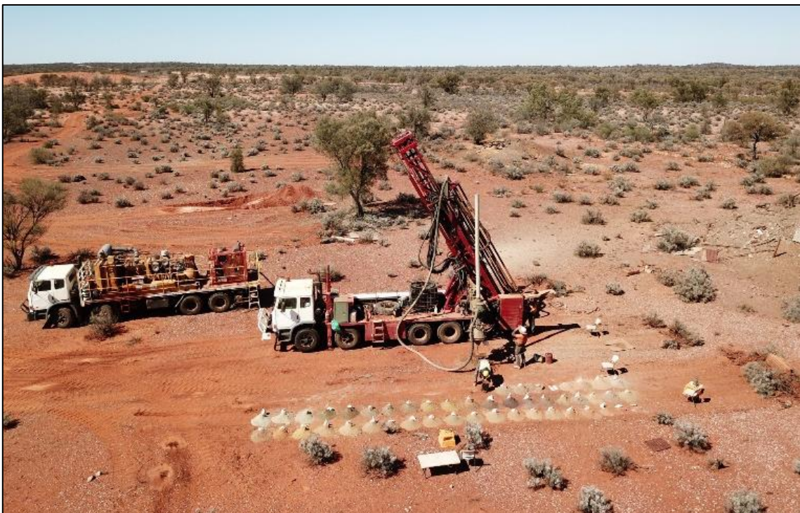
Anglo Saxon Gold Project, RC Drilling at Sulphide prospect ,Pinjin 2023.
