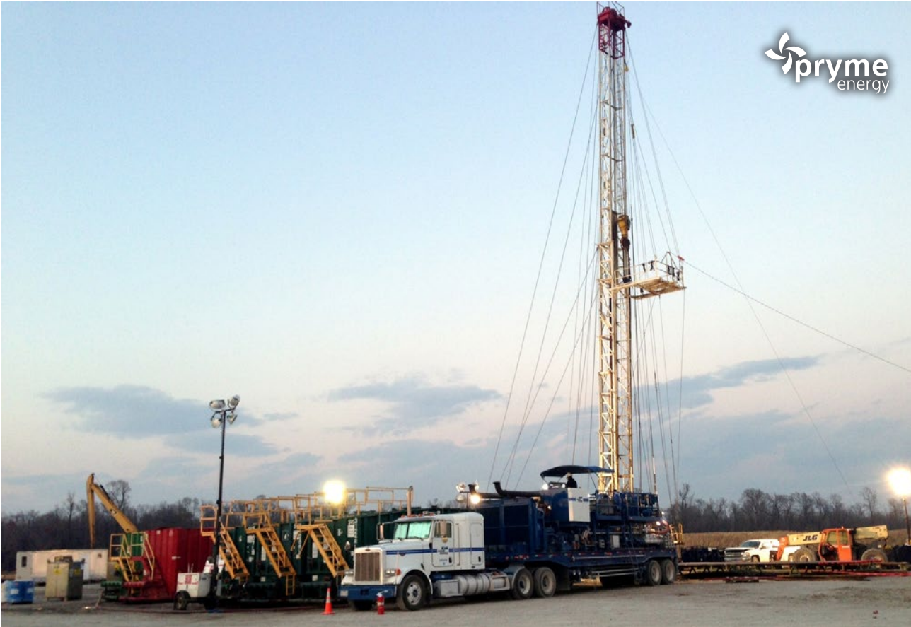
Work over rig running production tubing on the Rosewood Plantation 21H well
