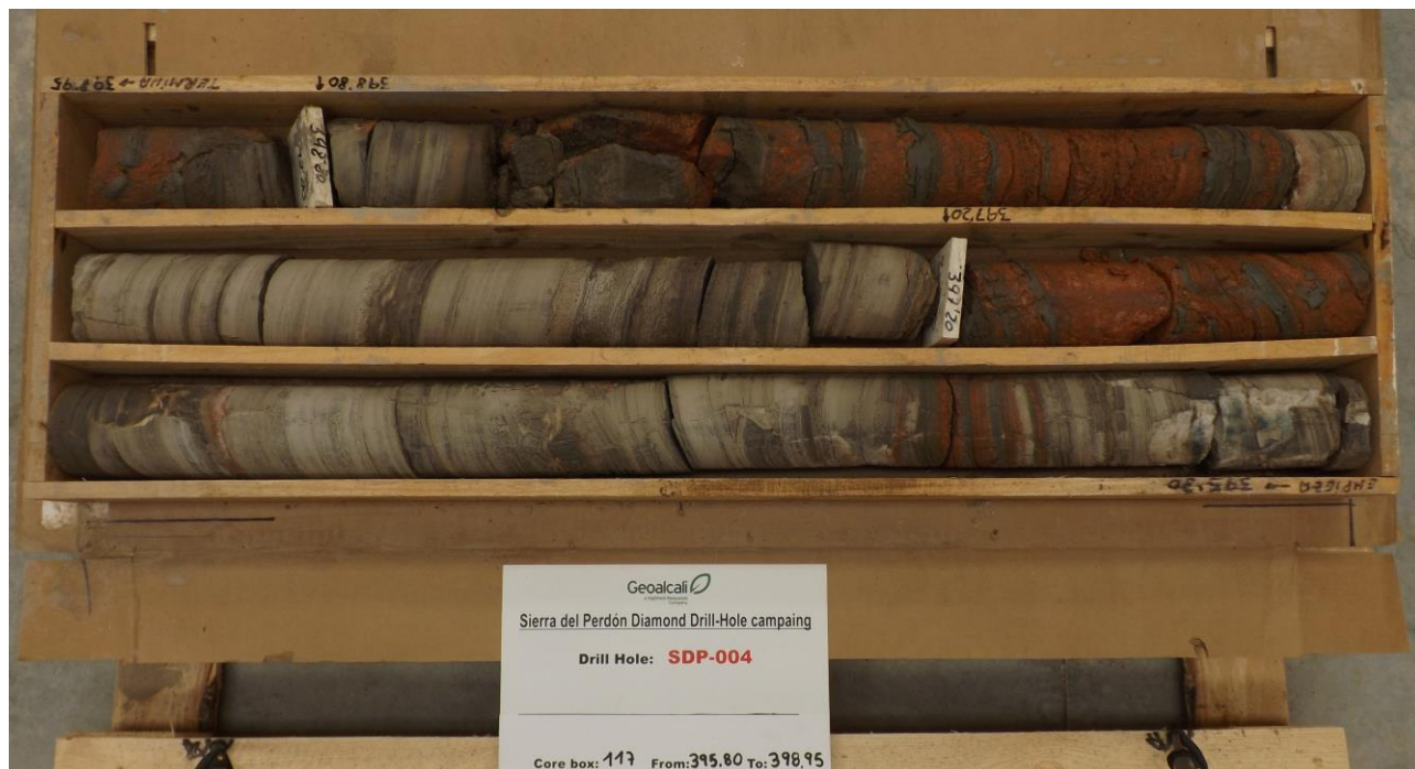
Figure 1: Core samples from initial drill hole on the Sierra del Perdón Potash Project (395.80 to 398.95m)
