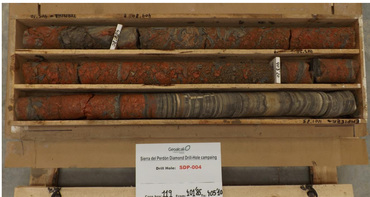
Figure 3: Core samples from initial drill hole on the Sierra del Perdón Potash Project (401.85 to 405.10m)
