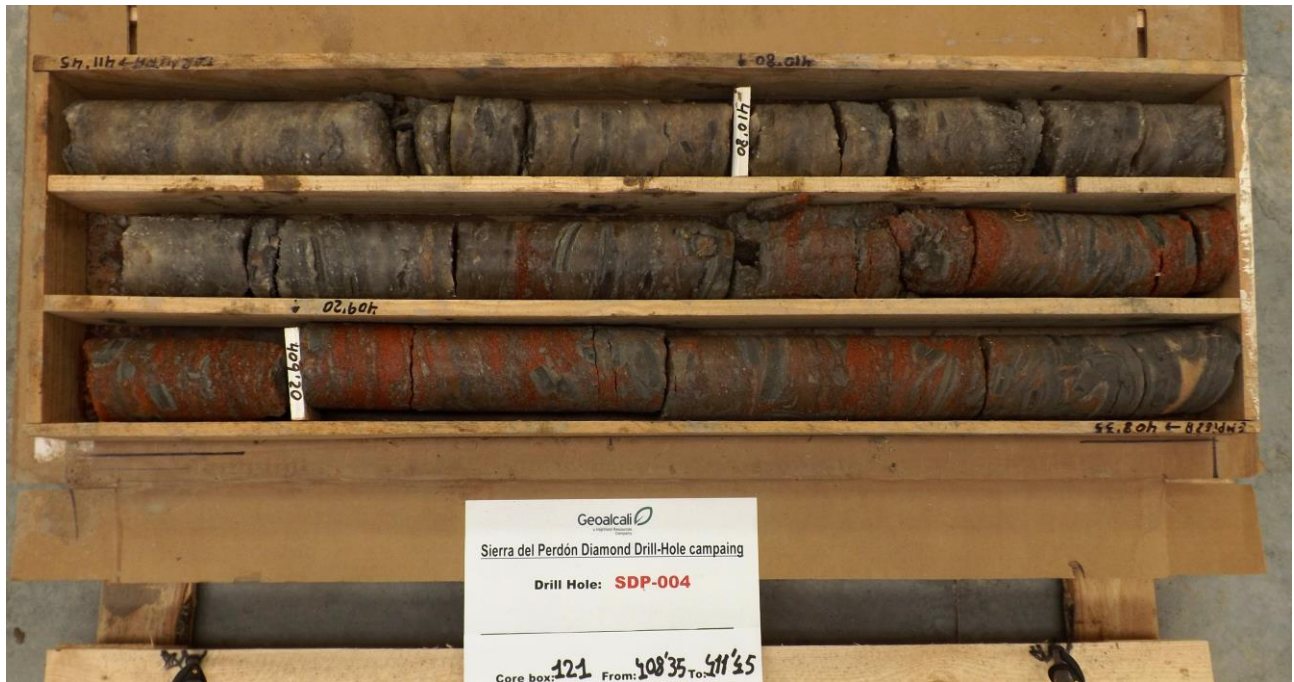
Figure 5: Core samples from initial drill hole on the Sierra del Perdón Potash Project (408.35 to 411.45m)
