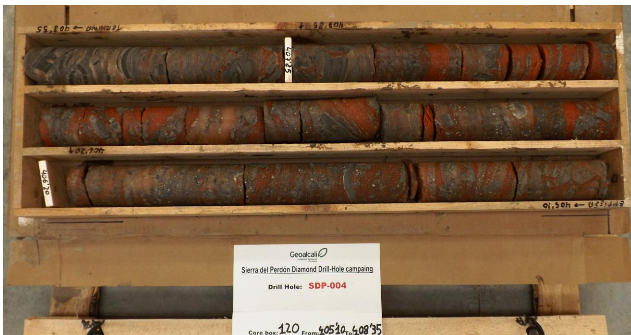
Figure 4: Core samples from initial drill hole on the Sierra del Perdón Potash Project (405.10 to 408.35m)
