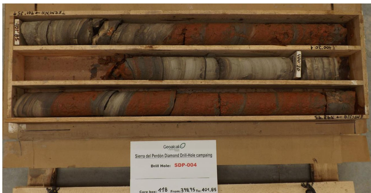
Figure 2: Core samples from initial drill hole on the Sierra del Perdón Potash Project (398.95 to 401.85m)
