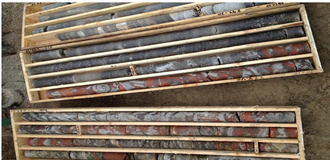
Figure 1: Photos of core samples in the field from DDH J13-07 showing potash mineralisation (red)
