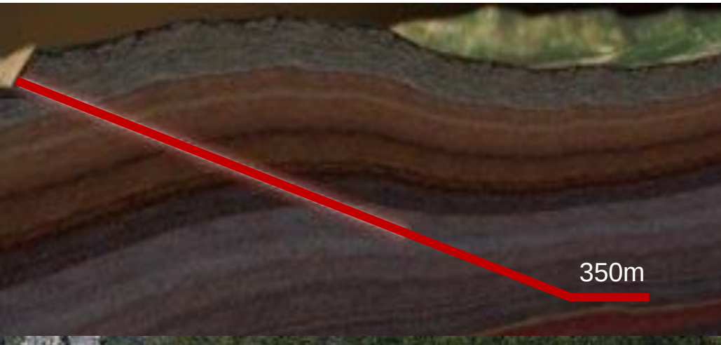
Decline access to shallow mineralization; underground Room and Pillar mining. No aquifers
