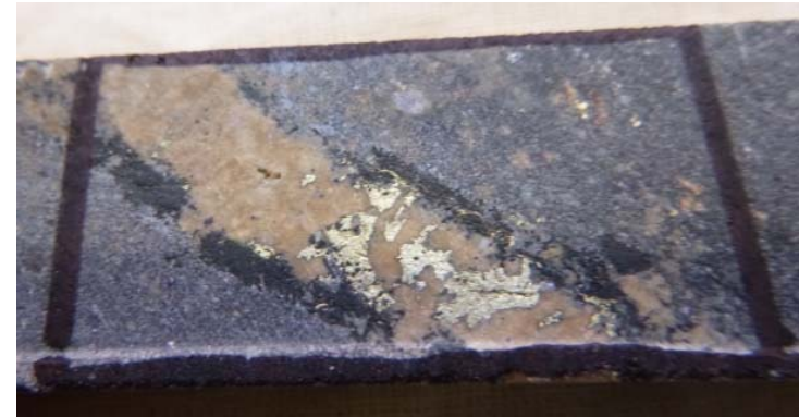
K-feldspar +/- albite vein 483.7 +/- 4.4 Ma monazite Po & Cpy later than feldspars B.Kimpton - 2018
