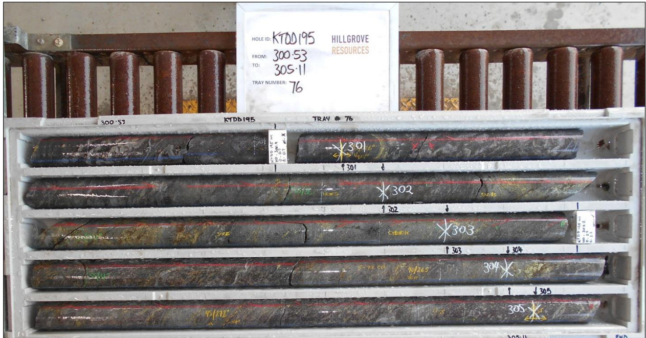
Figure 8: Core from KTDD195 (from 300.5m to 305.1m downhole) showing the silicious BCGS from Nugent
