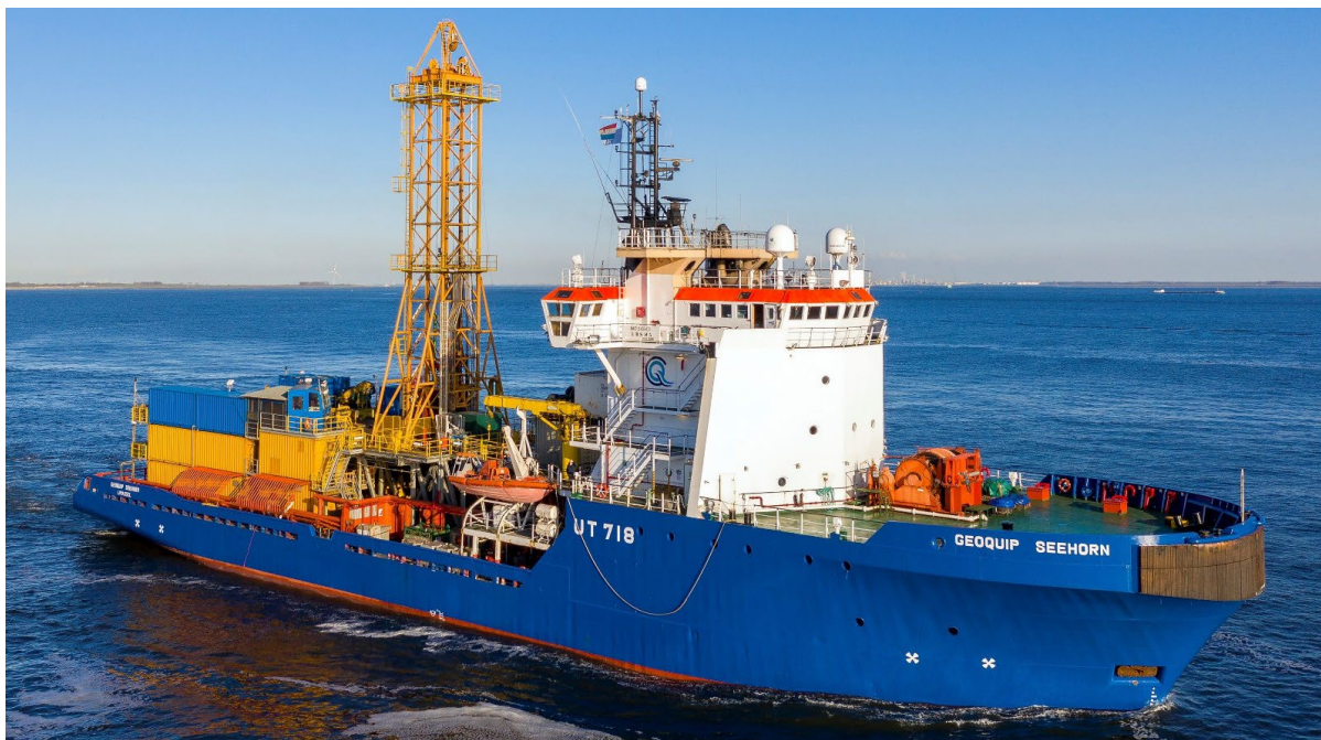
Figure 1. The Geoquip Seehorn DP2 vessel
