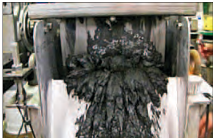
Photos 1, 2: HRL Testing ball mill (above) and magnetic separation (below)
