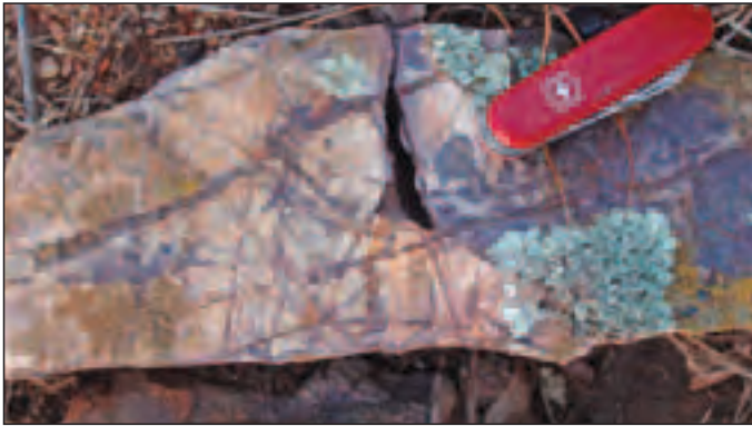
Photo 3: Hairline quartz stock work in siltstone (5.6ppm gold)
