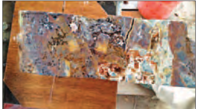
Photo 4: Gossanous (after sulphide), quartz-flooded breccia from Advene (Josephine Moulder) lode
