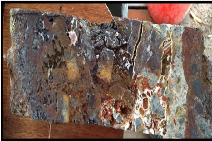
Photo 1. Gossanous (after sulfide), quartz flooded breccia JM lode
