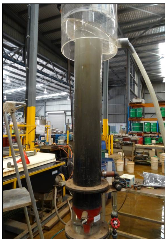
Photo 2 Hydroseparator with Hawsons material, Iron Ore Technical Centre, WA
