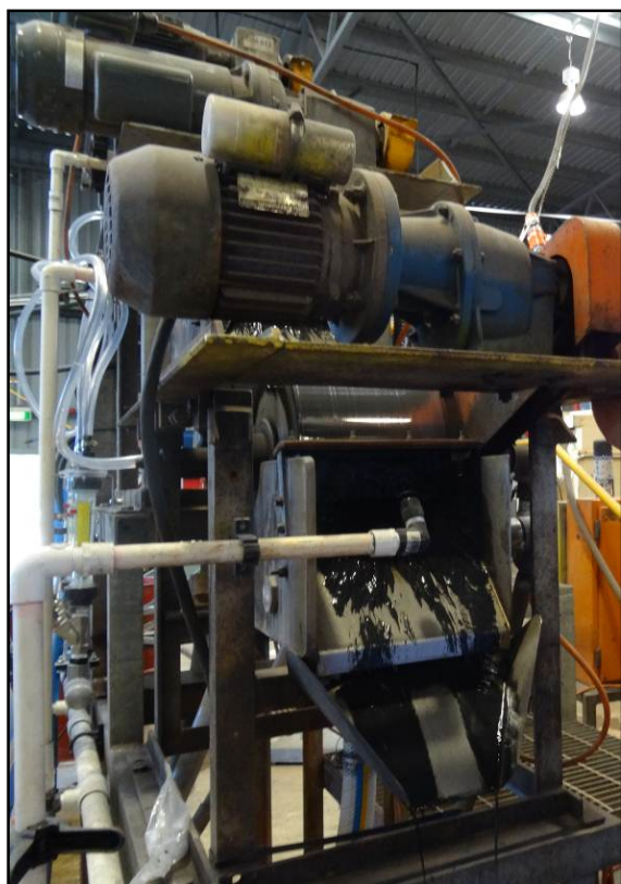
Photo 1 Pilot plant cleaner magnetic separator in action, Iron Ore Technical Centre, WA
