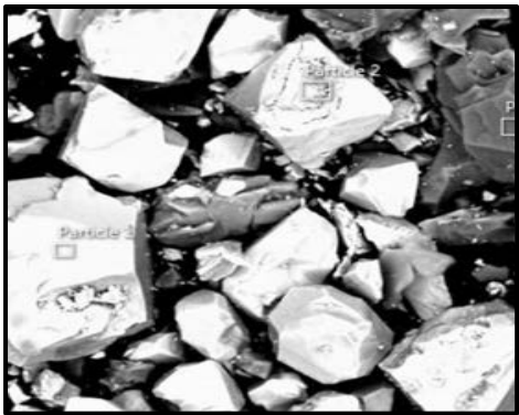
Elutriation removes free silica upgrade > 69%Fe
