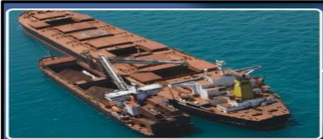
Iron ore concentrate transferred to ocean going vessels
