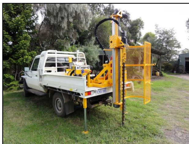
Figure 3: Helix Auger Rig will allow our team to sample a consistent soil horizon across areas of variable cover (up to max 20m). This will be used to identify drill targets on the southern extensions of the Tritton and Kurrajong VMS trends for testing in 2H12.
