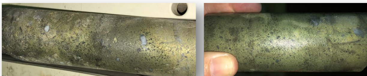
Figure 1: Photos of core from CORCDD090, the massive sulphide is dominated by copper-bearing chalcopyrite (assays are pending)
