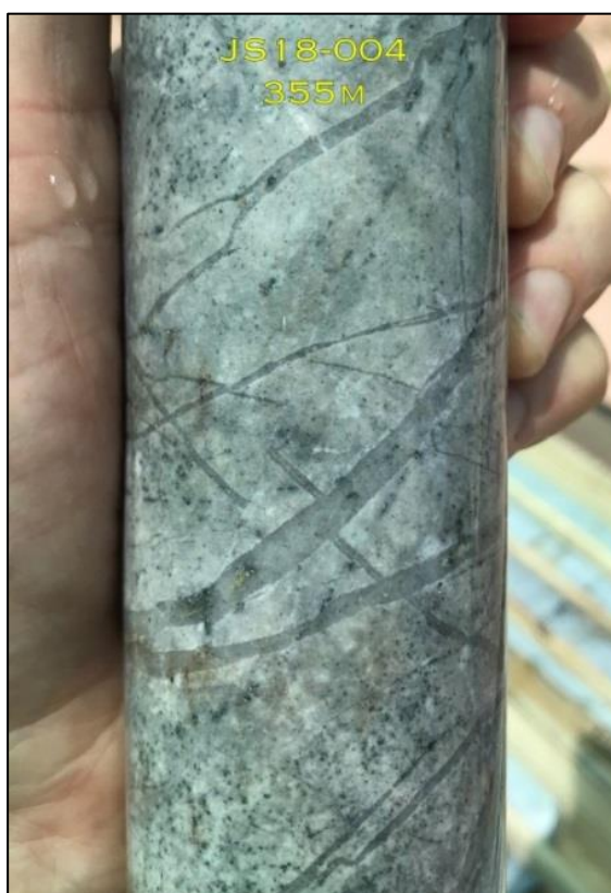
Photo 2 A. | Silicified dacite porphyry containing molybdenite-bearing A-type quartz veins (hole JS18-004, 355m). Assays awaited.
