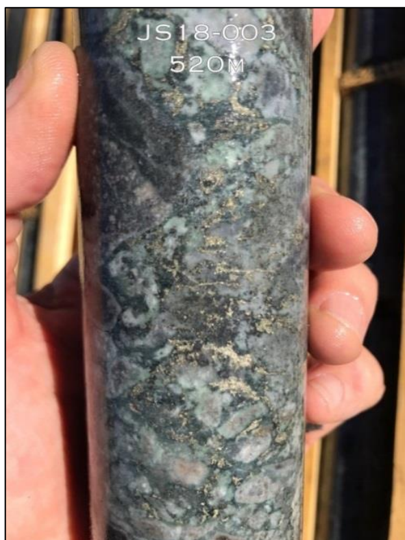
Photo 2 C. Hydrothermal dacite breccia with albite rims on breccia clasts and sulphide-bearing silica-chlorite matrix (hole JS18-003, 520m).
