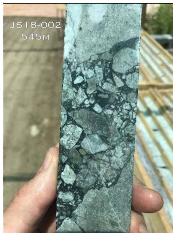
Photo 2 D. Sulphide-bearing hydrothermal dacite breccia with tourmaline matrix (hole JS18-002, 545m).
