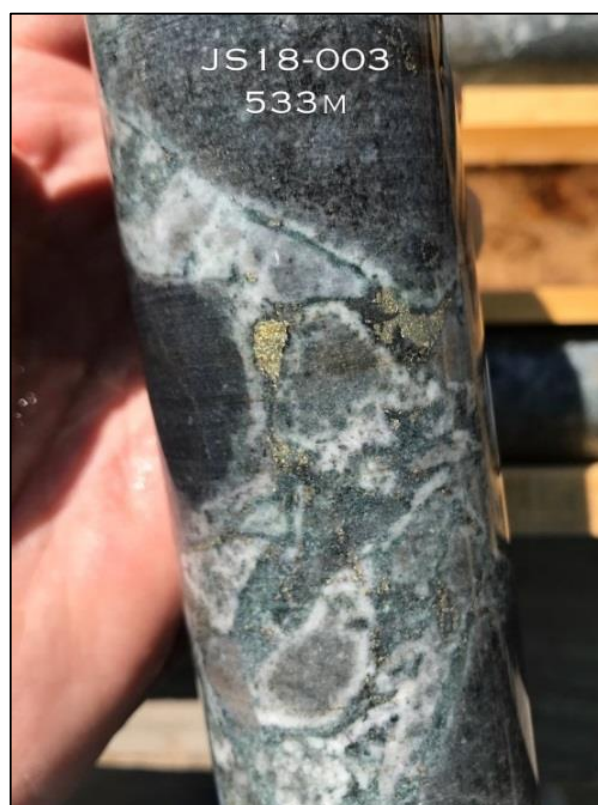
Photo 2 B. Hydrothermal dacite breccia with albite rims on biotite-magnetite altered breccia clasts and with a sulphide-bearing chlorite matrix (hole JS18-003, 533m).
