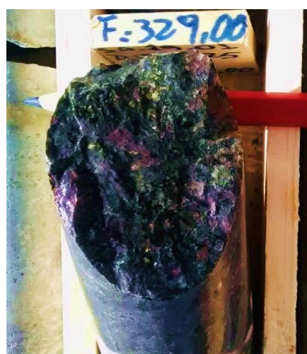
Photo 2: Traces of mixed primary sulphides (chalcopryite and bornite)* on fracture planes in altered andesite at 329m in Hole 1
