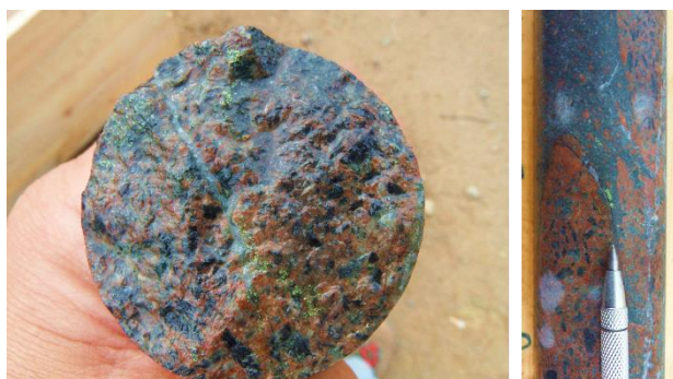
Photo 3: Traces of disseminated primary copper sulphides (chalcopryite)* in altered monzonite between 385-405m.
