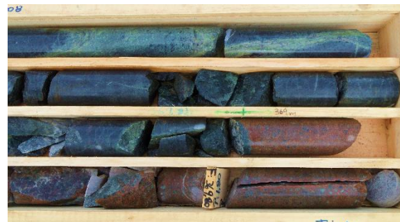
Photo 2: Traces of mixed primary sulphides (chalcopryite and bornite)* on fracture planes in altered andesite at 329m in Hole 1
