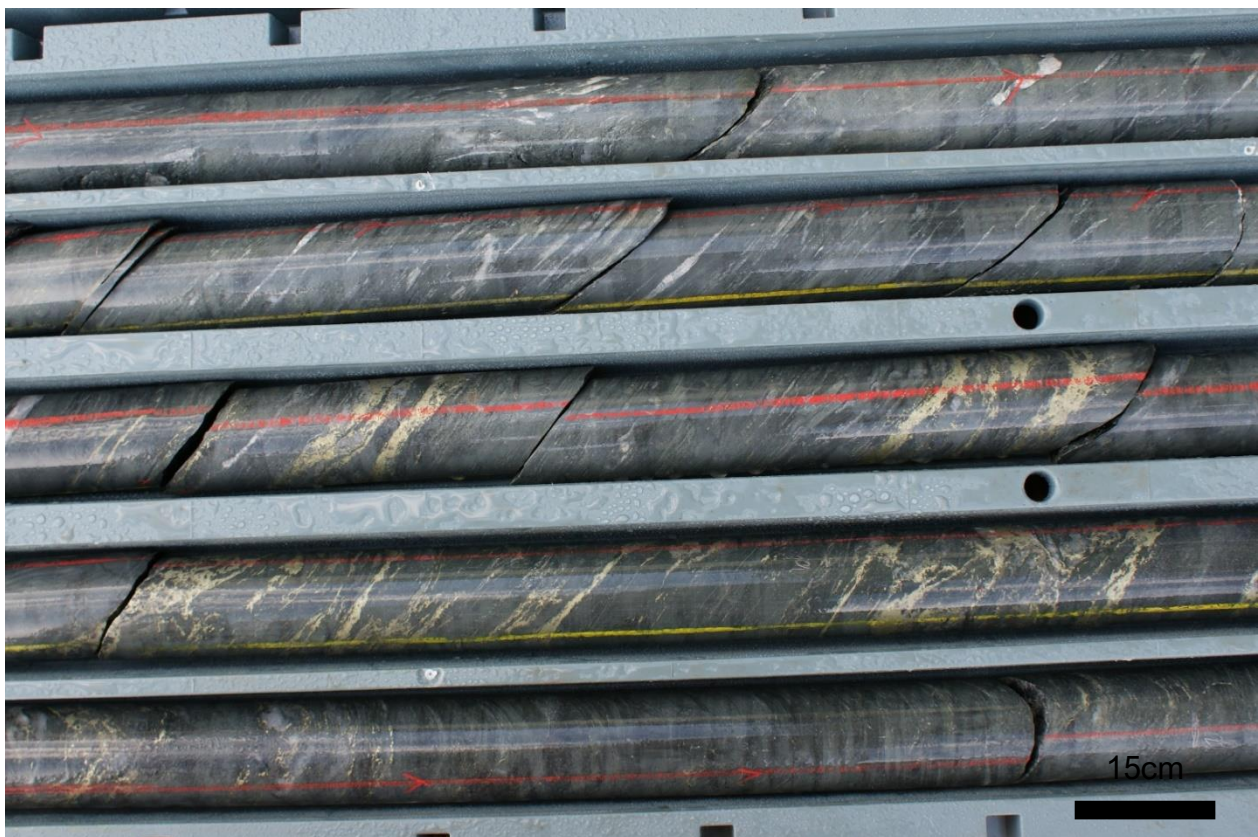
Figure 1: Disseminated and vein-fill chalcopyrite CAND001 ~278 metres downhole
