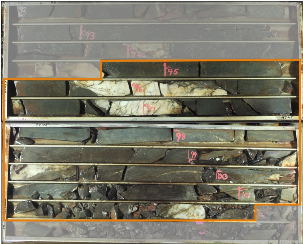
Figure 2: Mineralised intersection of 7.25m @ 3.09g/t Au from 94.75m in CMDD002 drilled in 2010
