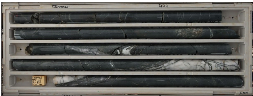
Figure 3: Hamelin's first diamond hole at Camel - TSD0005 (116m to 120.5m)
