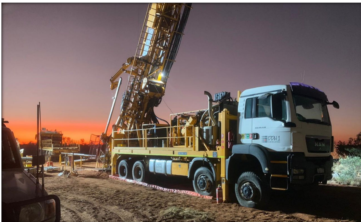
Figure 1: DDH-1 diamond drill rig operating at the West Tanami Gold Project
