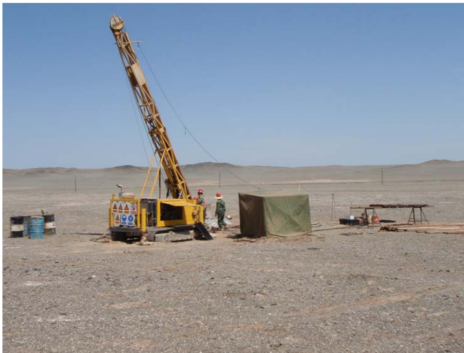
Fig 2 Diamond Drilling at Da Hong Shan
