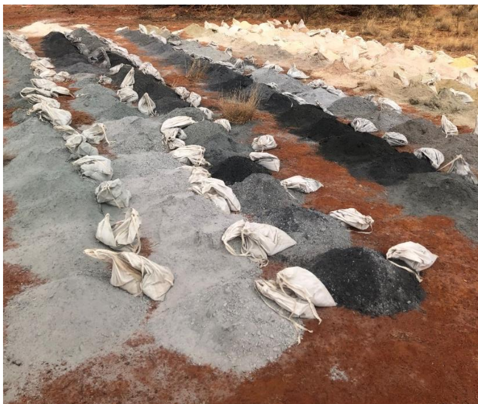
Figure 5. Target 4 – Drill chips from BWSRC0035 showing the prospective sulphidic unit
