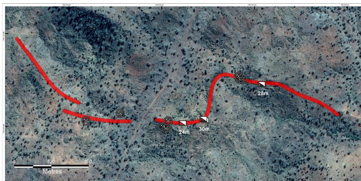
Figure 10. Lakeview prospect showing shafts (with depth) and the schematic lode position
