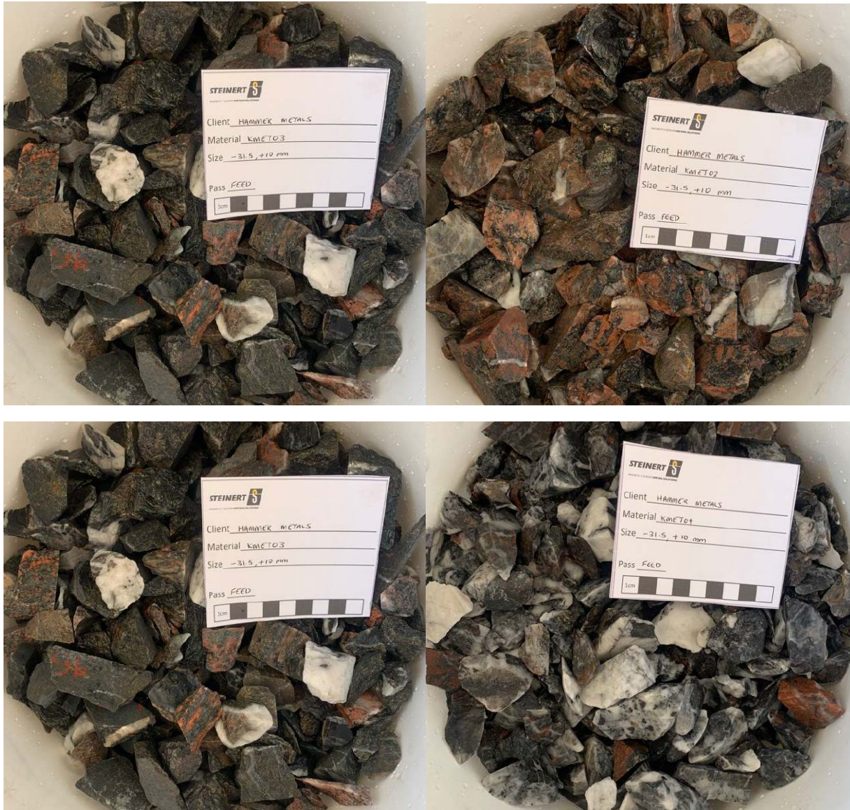
Figure 4. Examples of trial samples KMET01 (top left), KMET02 (top right), KMET03 (bottom left) and KMET04 (bottom right). Samples 1 through 3 are from the Cu-Au domain and were amalgamated. KMET04 was from the Mo-Re domain and was run separately.
