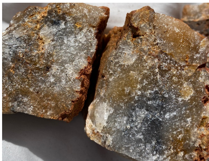
Figure 4 – Sample MW2211_68. Sulphidic Quartz Vein. This specimen analysed at 0.35g/t Au, 341g/t (or 10.96oz) Ag and 0.25% Bi.
