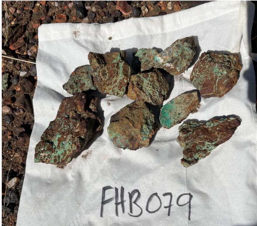
Figure 11. Chalcocite and malachite mineralisation – Sample FHB079 – Laboratory assays of 24% Cu and 0.14g/ Au.
