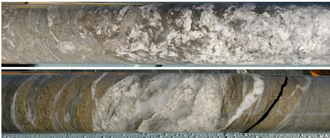
Figure 3. Top: Details of the quartz–carbonate–pyrrhotite-+/- pyrite, chalcopyrite breccia zone within the upper mineralised zone. Note the strongly bleached host rock to the left. Bottom: quartz - carbonate veins in the lower alteration zone (421.2m to 422.7m) showing brown alteration selvage. The veins contain trace pyrite and pyrrhotite. The brown alteration zone grades into a pale grey bleached alteration zone.
