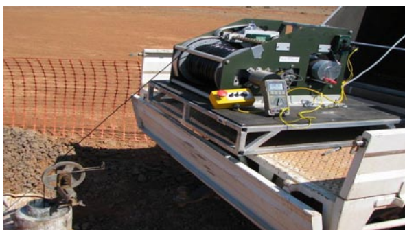
^ Fig 6: Temperature Logging in exploration well Balrog 1, Parachilna Project. Temperatures logged are combined with thermal conductivity measurements to derive heat flow values from each well.
