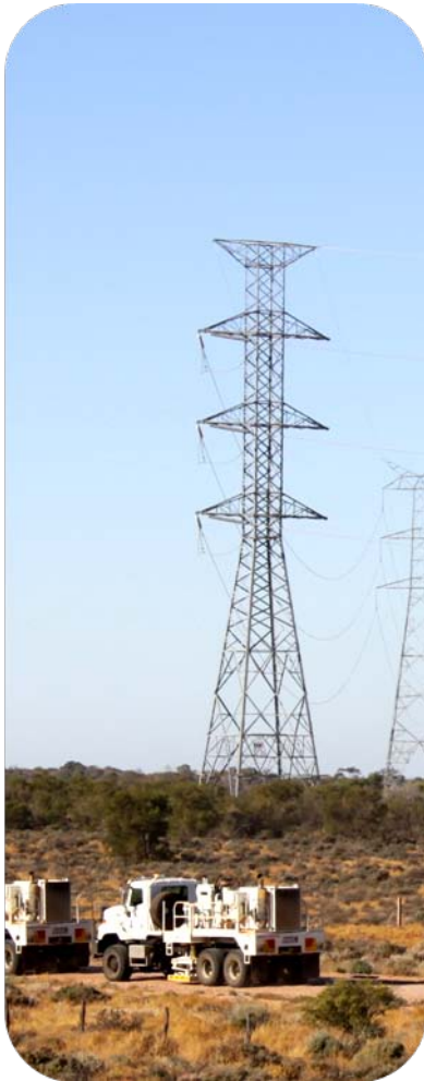
Terrex's 'bird-wagen' MARK IV off-road carrier with HEMI 60 vibrator on Parachilna – Leigh Creek 132KV line.
