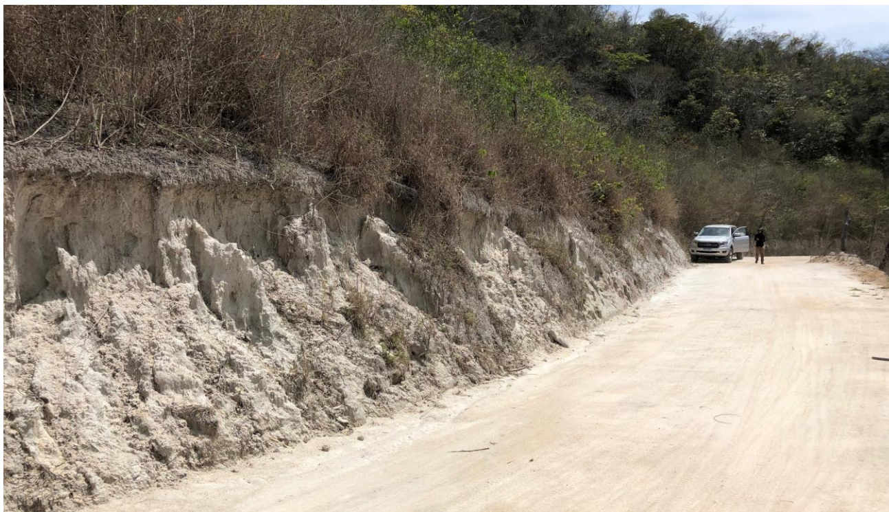
Figure 5: Highly weathered coarse quartz rich road cut at Carai which extends for 80m and sits below artisanal mine workings.
