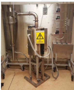
* Hazer's Fluidized Bed Reactor
