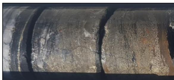
Figure 1: Claypan FMDD0040 ~140m, sulphidic zone associated with SCT/BIF.
