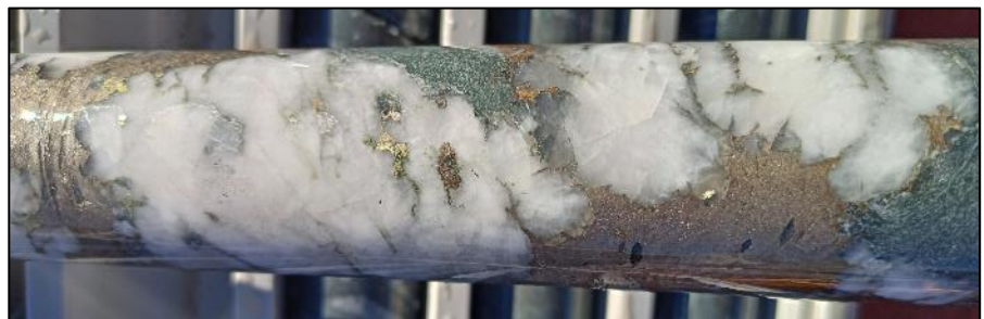
Figure 1: FMDD0047 ~231m, sulphide bearing quartz vein with pyrrhotite, pyrite, arsenopyrite and chalcopyrite hosted within andesite volcanics.
