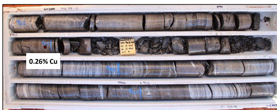
Figure 5 0.26% Cu (2,625.35 ppm Cu) returned from single pXRF data point at 942.99m; within a laminated shale unit. pXRF data was collected at systematic 0.5m point intervals, independent of geological boundaries.
