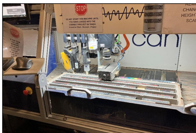
Figure 2 pXRF and ASD data collection on whole core using BoxScan at Galt Mining Solutions.
