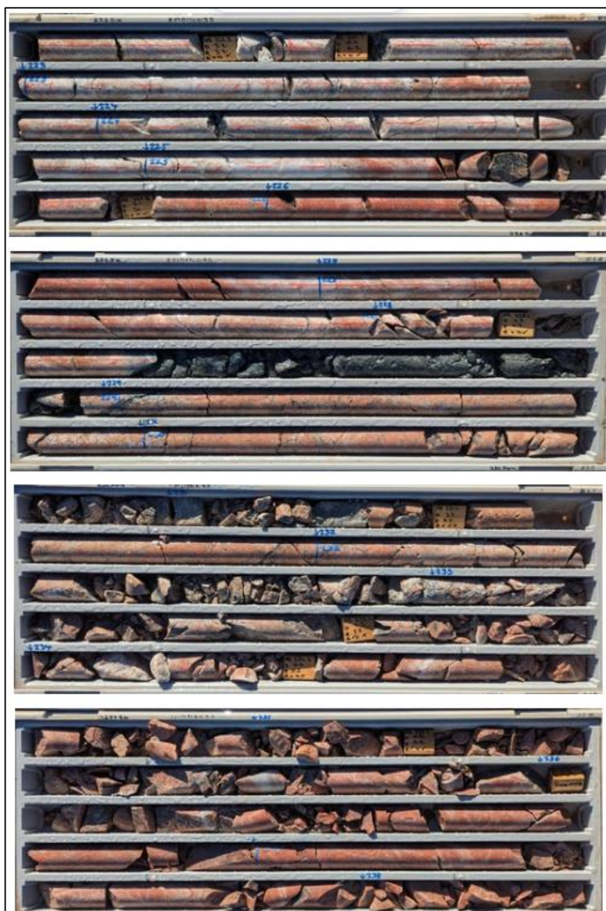
Figure 5 Diamond core tray photographs (core blocks 222.21m to 238.4m), showing the Gander Fault intersected by drillhole FMDD0058. The quartz syenite porphyry - monzogranite host rock exhibits progressively increasing carbonate-silica alteration towards the fault zone, which comprises an approximately 25m-wide interval of intense brecciation (broken core), fault gouge and sheared lamprophyre.*
