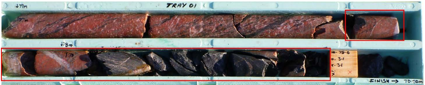
Figure 3: Intersection of 6.3 g/t Au, 1.76 g/t Ag in THDD065
