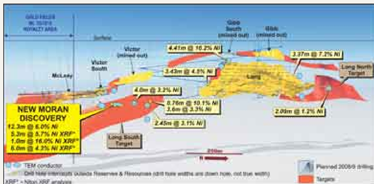
Figure 2: Long Nickel Mine - Longitudinal Projection Showing Target Areas, TEM Conductors, Significant Intercepts Outside Current Resources and Reserves and Proposed 2008/9 Exploration in Light Blue
