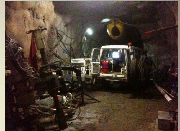
Underground Down hole TEM surveying
